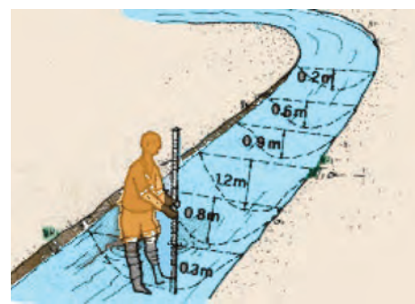
Fig. 6-5 Area of Flow (Depth & Height)
