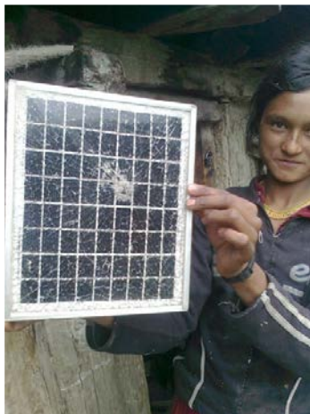
Fig. 4.2: An Example of the Damaged Module
